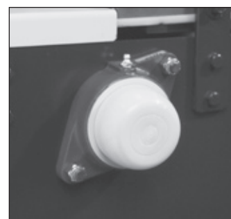
Safety end caps protect against rotating stub shafts.
